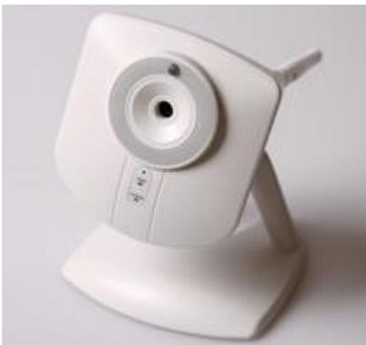
Inexpensive IP (Internet Protocol) cameras have revolutionized security and communications by showing live video from one location to another via the Internet. Most of them work via Wi-Fi, and some are designed for outdoor use.
