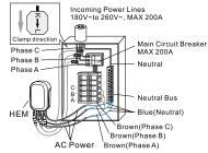
To perform the electrical installation for your Home Energy Meter (HEM), utilize the previous images to determine the phase version of the HEM and to also illustrate the following
