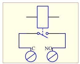
Schematic outlines of how the relay outputs are implemented internally
