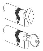
To mount the Danalock on a door with an euro cylinder you will have to exchange it.
