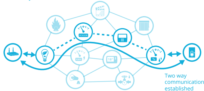
Figure 3. DOOR LOCK IS AWAKE - Packet is delivered and acknowledgement of delivery is returned to controller
