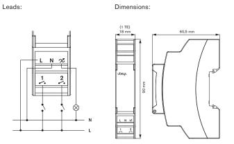
The power switch S1-R retains its switch position when disconnected from power. The switch position is undefined by delivery; i. e. the switching output can be conductively connected to the phase L!
