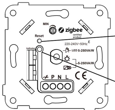
Step 1: Press and hold reset button for over 5 seconds.
