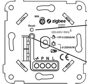
Step 1: Press the reset button 5 times.
