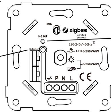
**Step 3:** Double Press the reset button to activate the network pairing mode (The blue indicator light is flashing), network pairing mode will last for 15 minutes once timeout repeat this step.
