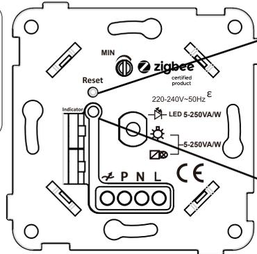
Step 1. Press the reset button for 6 times to enable the device to setup a zigbee network.
